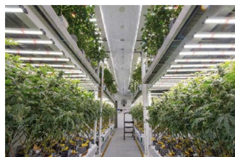
Figure 3. Example multilevel, mobile racking system in a commercial grow.
